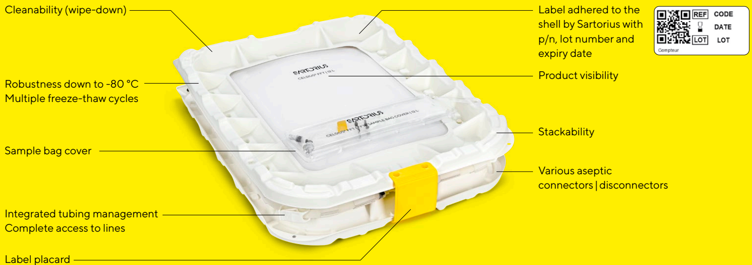
Figure 2: Key Features of the Second Generation of Celsius® FFT|FFTp Containers
